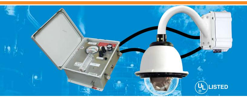
UL Class 1- Division 2 Certified, Videolarm's PurgeDome Explosion Proof camera system provides a highly effective solution for monitoring in explosive/hazardous environments. Operating on a supply of compressed air or inert gas, the PurgeDome system regulates the pressure within the sealed camera enclosure protecting it from extremely hazardous fumes or gases, which could ignite in a violent explosion.
